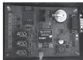
GSM MONITORS AND CONTROLS JVA ENERGIZERS USING A CELL PHONE
