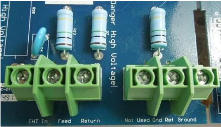
Description of high voltage terminals (left to right)
