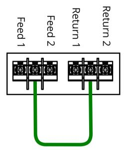
Arm the Z28 once again, after 3 pulses (unless you configured it otherwise) the unit should go into alarm as the fence will appear to be cut. Check that any sirens, strobes or relays correctly activate as you expect.
