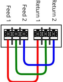
Power the Z28 and then Arm it. The unit should begin pulsing and not show any alarms. Disarm the Z28 and remove the fence cable as shown in the picture below.
