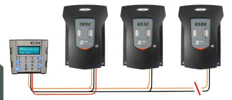
By disconnecting each Z-Series Energizer in turn from the keypad bus (shown in the above diagram) you can check to see how each Z-Series device behaves under communications failure (comms fail) conditions. This way, you can test to see that the relays have been configured correctly for comms fail. Once you are satisfied that each Z-Series device is configured correctly you can begin to wire them to the real fence.
